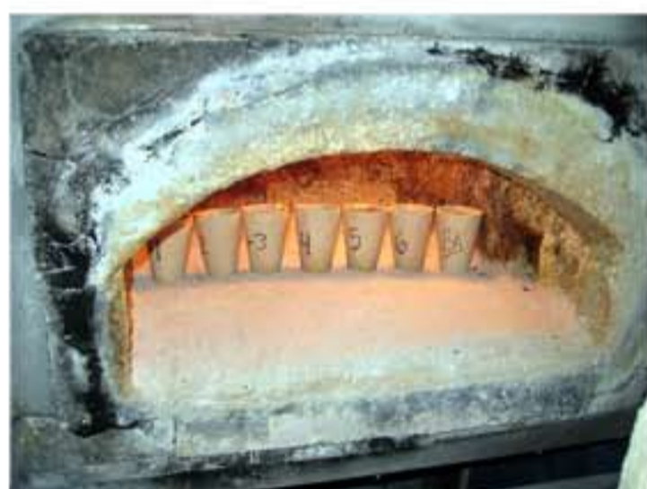
Photo 4: The furnace requires cleaning and should be operated at about 1100 C.
