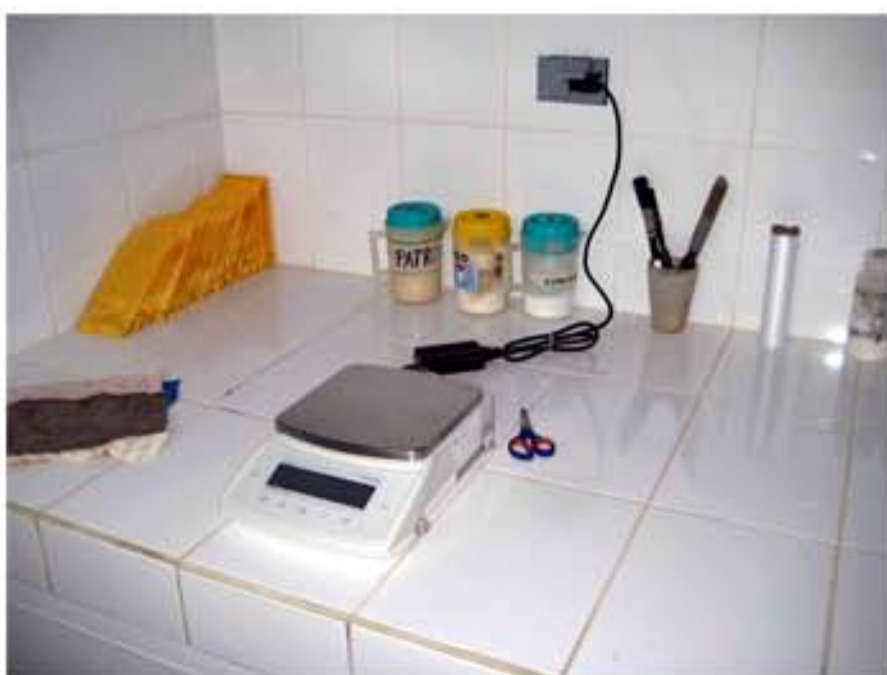
Photo 5: Fire assay balance has never been calibrated or certified. The lab does not have a set of certified standard weights.
