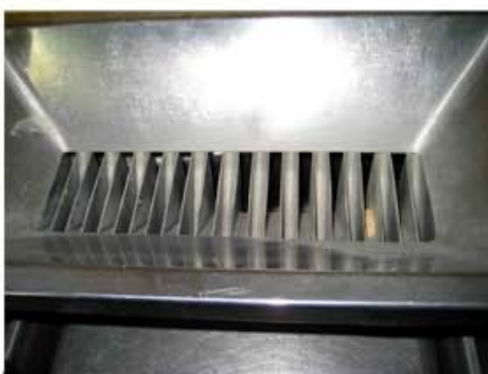
Photo 3: There is grease on the splitter, originating from the crusher. This is therefore in the sample and the pulverizer. Gold can be lost due to sticking.
