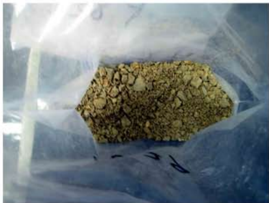
Photo 2: This is not a dry 85 % -2mm crusher product. The sampling precision will not be optimal because of the large pieces.
