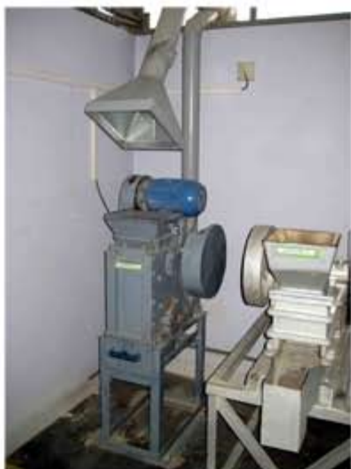
Photo 1: The crusher requires cleaning of grease from the bearings more frequently. The jaws are set too far apart, producing coarse material before splitting.
